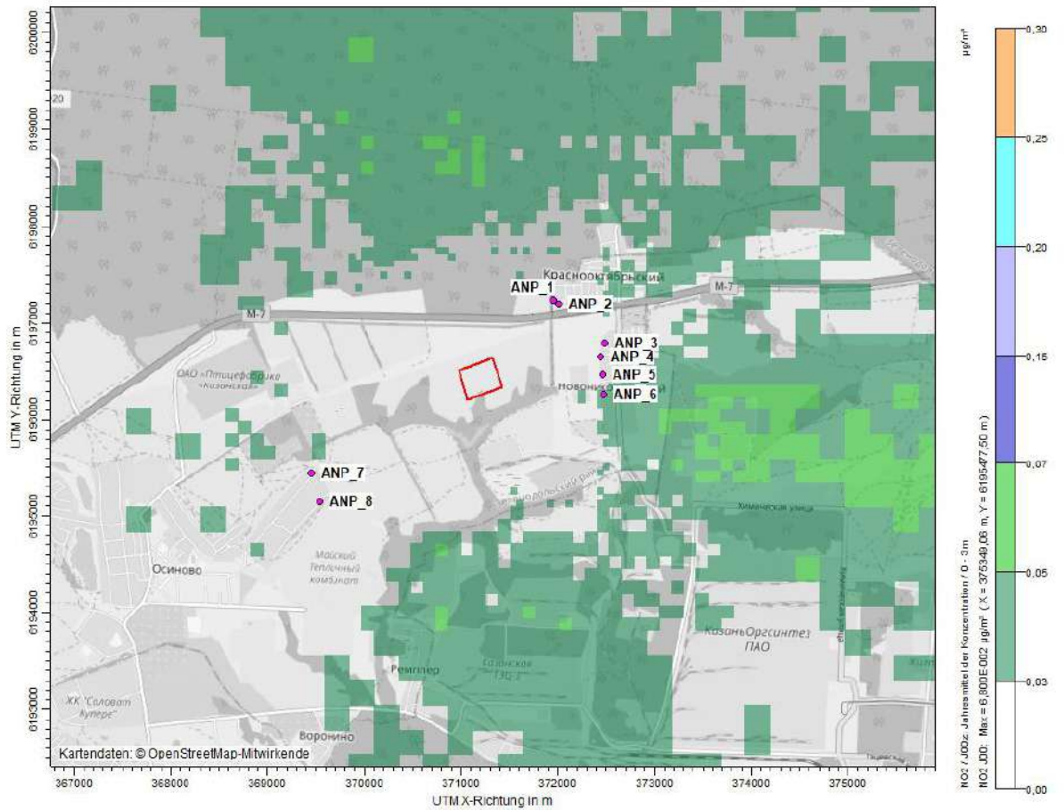
Figure 5. Annual average additional load/contribution of the waste incineration plant J00 in \mu\text{g}/\text{m}^3 for Nitrogen dioxide. Monitoring sites are shown as pink dots; waste incineration plant yard shown as red rectangle
